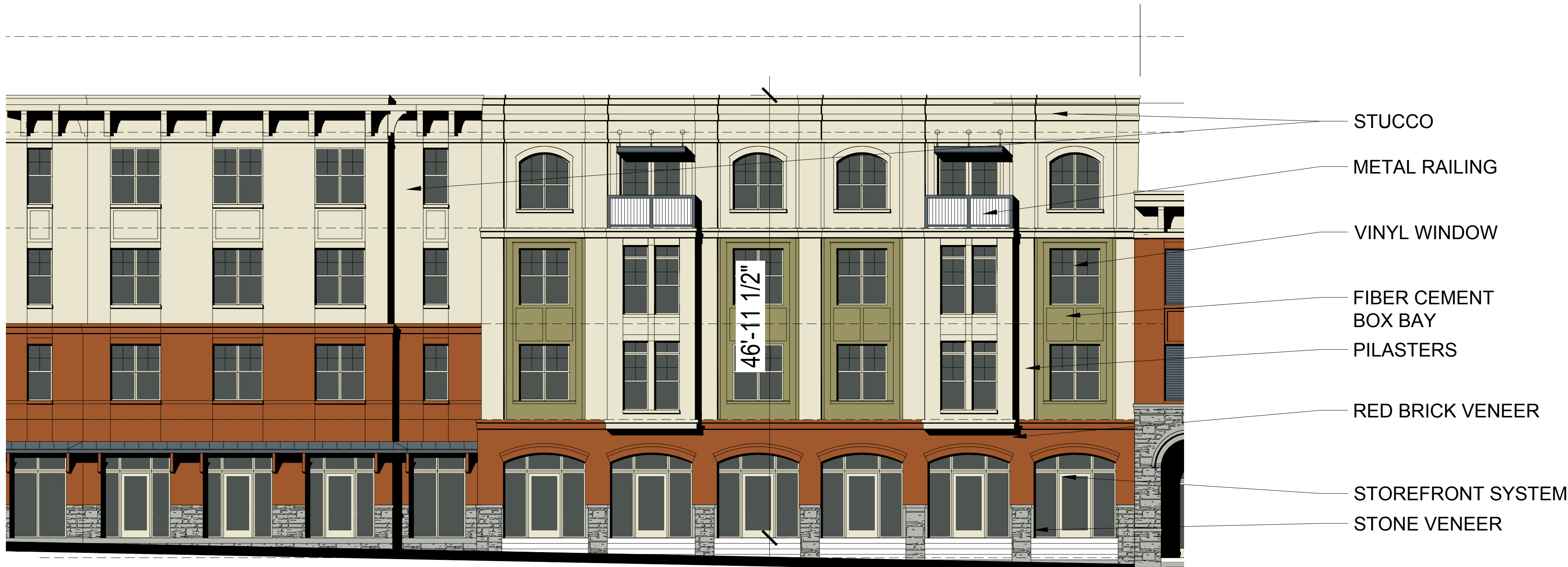
BUILDING 1B POPLAR GROVE ROAD FACADE
