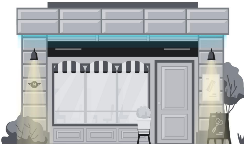
Figure 27.02.02 (D). Tube lighting recessed, thus making it shielded.
