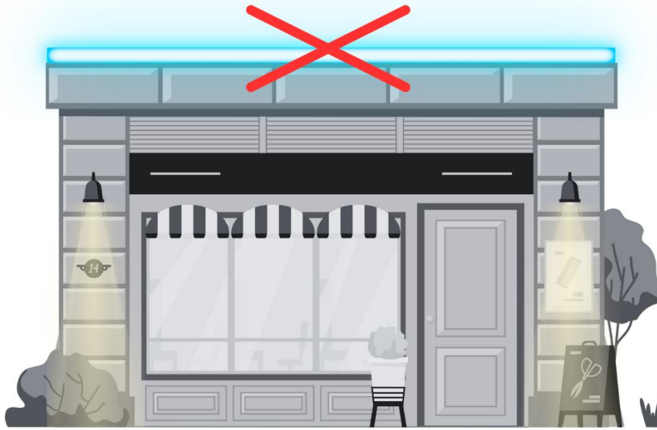
Figure 27.02.02 (D). Unshielded tube lighting prohibited.
