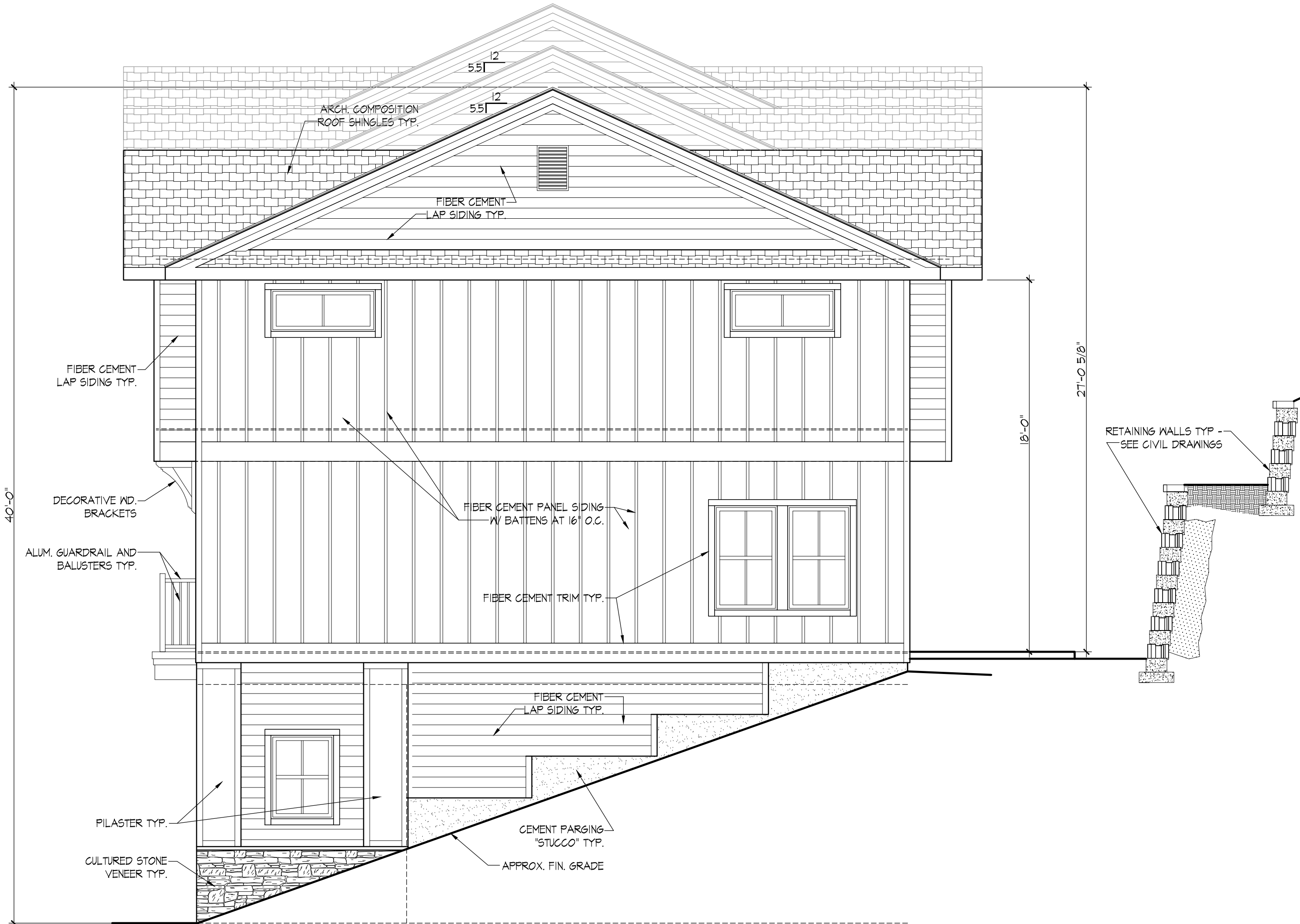
CONCEPTUAL RIGHT SIDE ELEVATION - BUILDING 200 SCALE : 1/4" = 1'-0"
