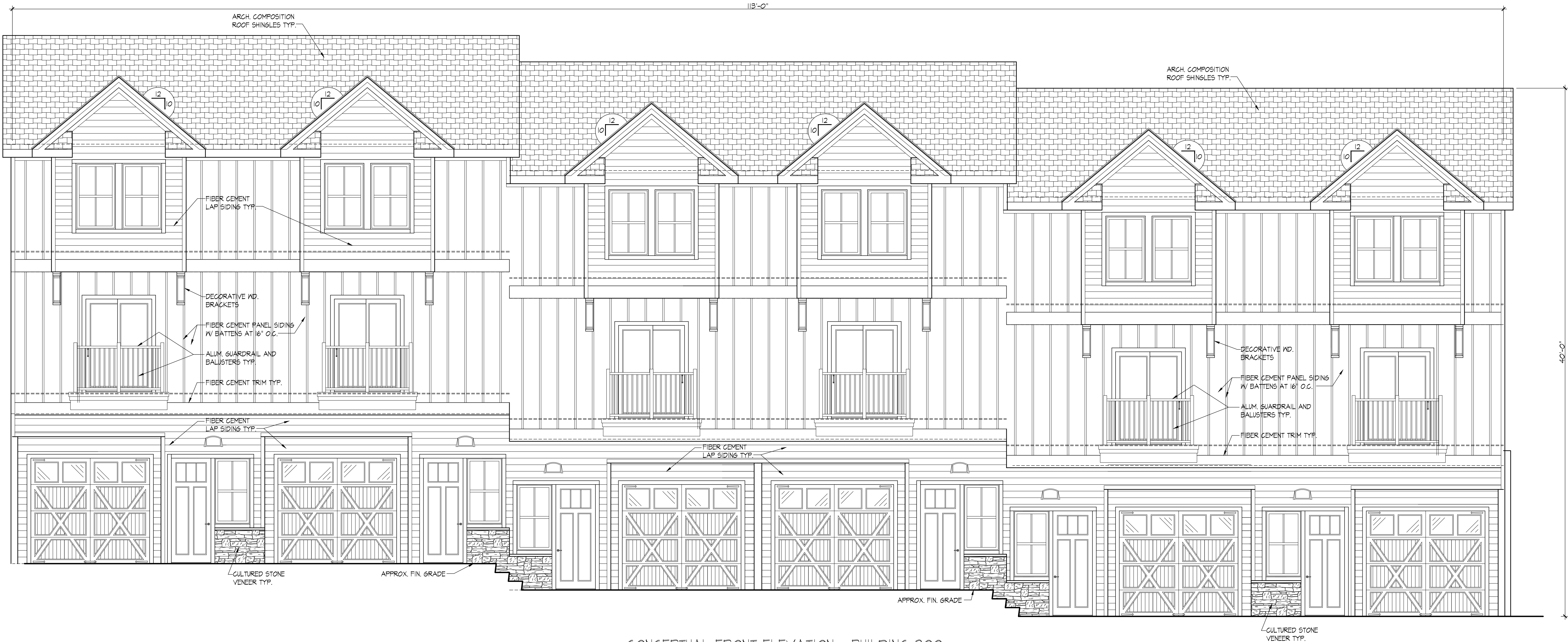
CONCEPTUAL FRONT ELEVATION - BUILDING 200 SCALE : 1/4" = 1'-0"
