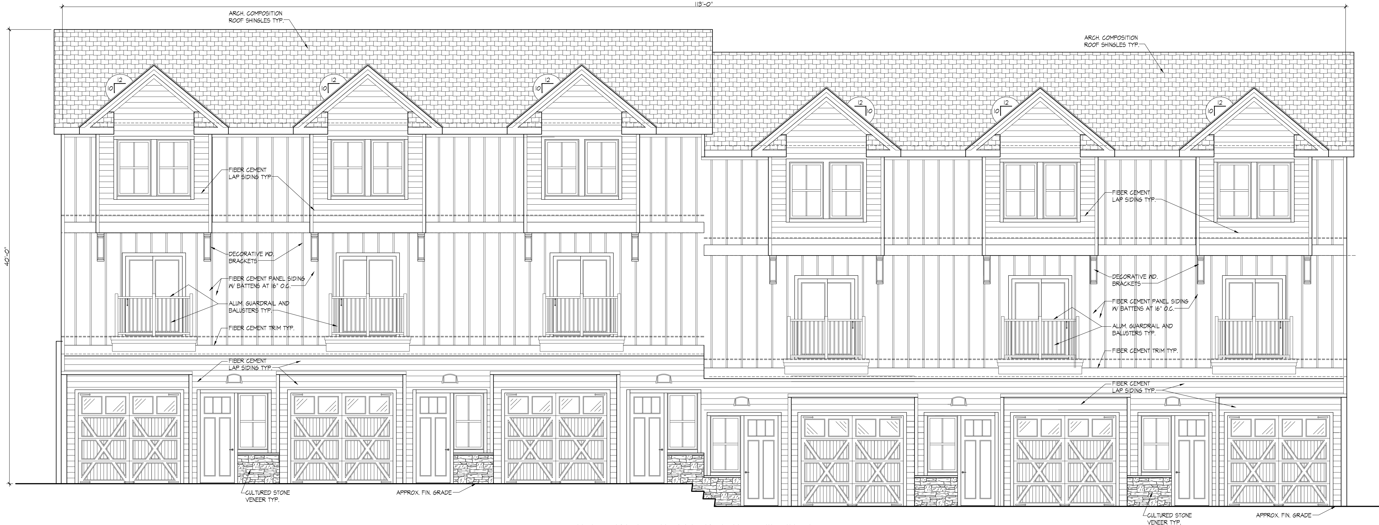
CONCEPTUAL FRONT ELEVATION - BUILDING 100 SCALE : 1/4" = 1'-0"
