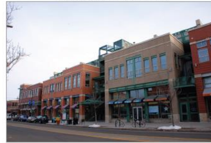
Figure 5.7.E(3)a: Example of Front Façade Offsets
