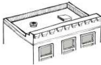
Roof parapet hides flat roof plane and utility equipment
